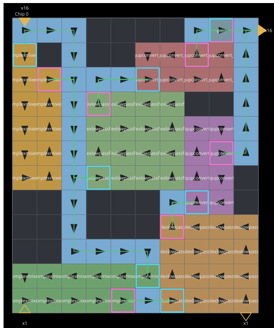
Figure 3. The Weaver SSB transceiver, a dense hand-placed design occupying most of the 120-cell array. Both the transmit and receive chains are resident at once: complex mixers (orange and green), complex low-pass filter banks (green and tan), and IQ up-conversion (red and purple), with routing cells (blue) threading between them. This is the layout that produces the SSB row of Table 3.
